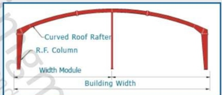
Multi Gable Maximum practical module width = 80 m
